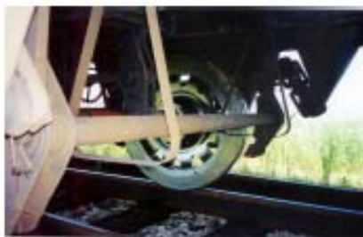
Perforated AD860F with ring damper, (ABB/CAF manufacture)
