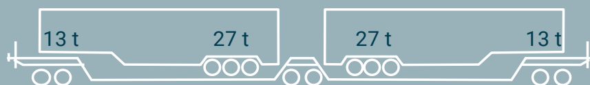
Figure 3: Loading plan for an articulated pocket wagon (e.g., TWIN) with two semi-trailers and maximum load capacity.
