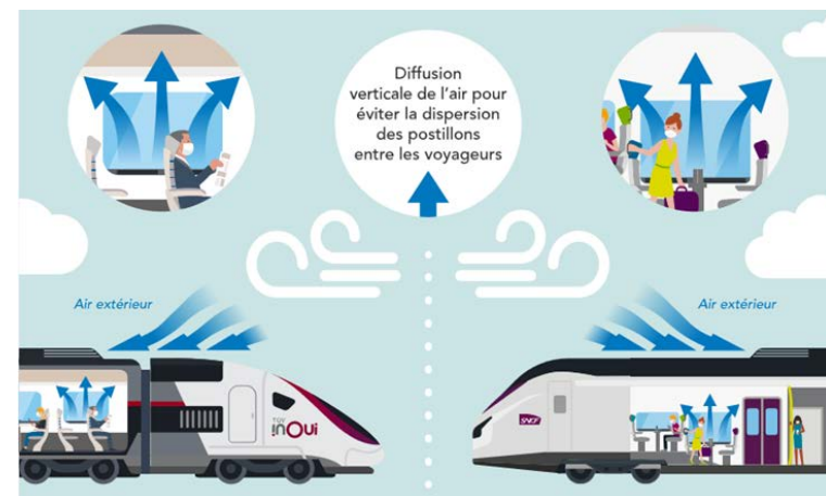
Figure 1: Figure from SNCF demonstrating how the air circulates in their ventilation systems on board TGV and other trains
